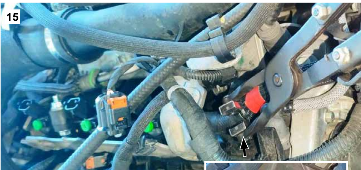
15) Insert gas pipe and fix the clip
