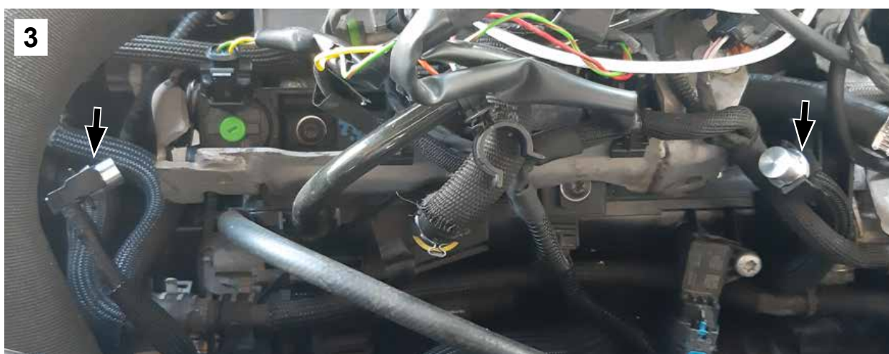
3) Remove rail water pipes and put the plug.
