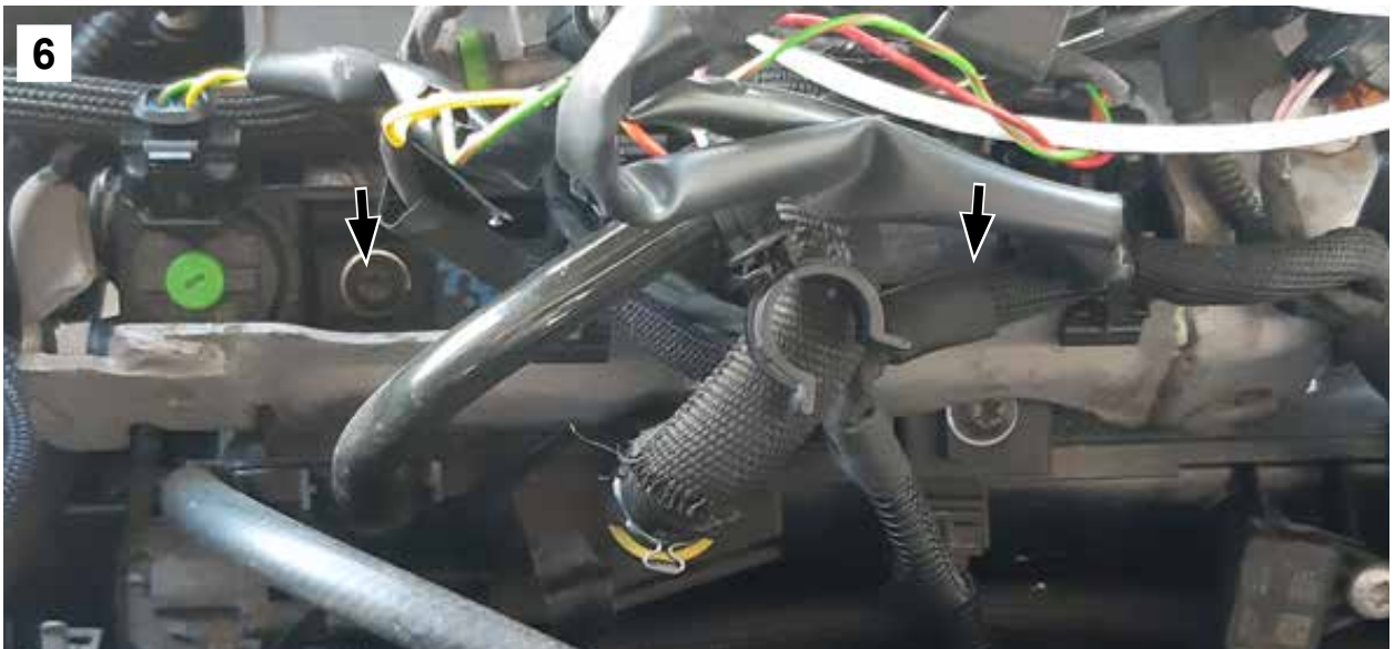
6) Unscrew the rail fixing bolts/nuts.
