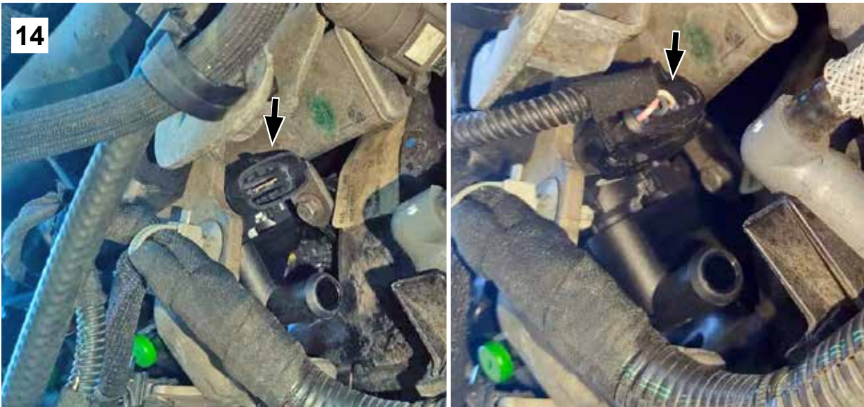
14) Insert P-T gas connector.
